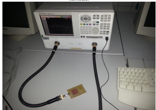
Figure 4. Antenna connected to network analyzer for measurement in laboratory.
