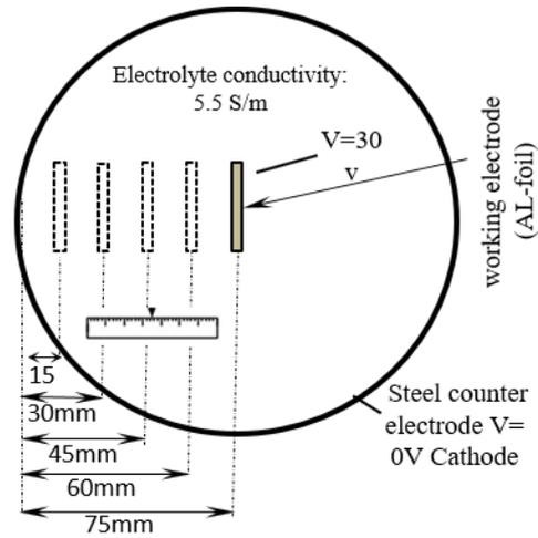
Figure 1. View of the 2 D. model domain and boundaries representing the sample placed in different distances from the counter electrode in the electrolyte.
