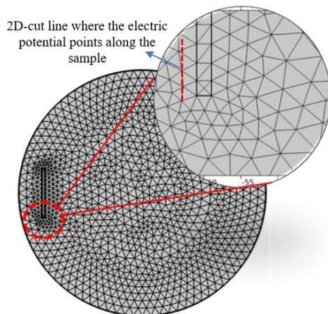
Figure 2. Meshing of the boundaries on the sample (anode)/electrolyte boundary.
