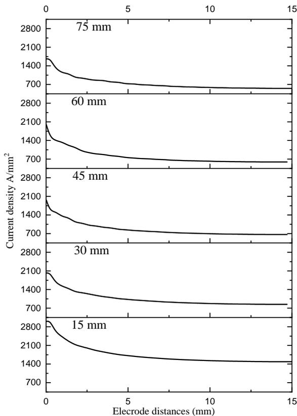
Figure 5. Simulated current density distribution along the surface of the working electrode.
