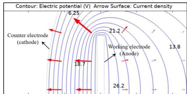
Figure 4. Modelling results of electric potential [V] and current density [ $A/m^2$ ] distribution respectively as contour and arrow lines
