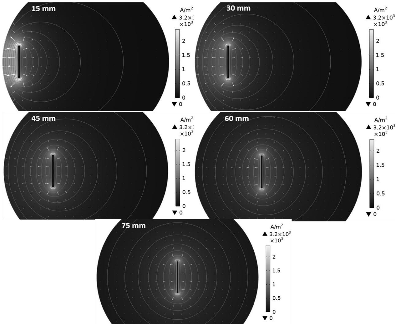
Figure 3. COMSOL modelling results of current density distributions ( $A/m^2$ ; surface and arrows) on the surfaces of anodes for different electrode distances between 15 and 75 mm.
