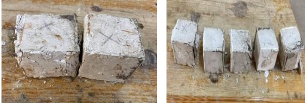
Figure 16. Specimens of root fibers (left) and remaining fibers on different sieve diameters after failure.
