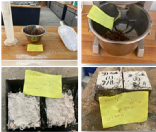
Figure 3. Preparation specimens of gypsum reinforced by date palm fibers.
