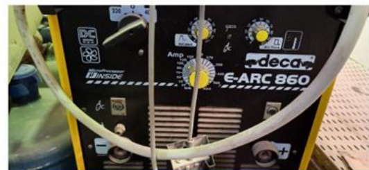
Fig 1: DECA E-ARC 860 DC welding machine used in the experiments
