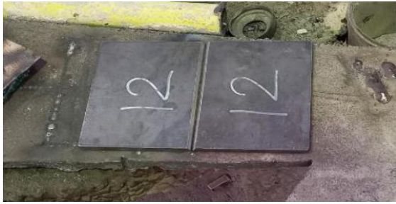
Fig.2. prepared low-carbon steel specimens prior to welding, showing the joint configuration used in the experimental work
