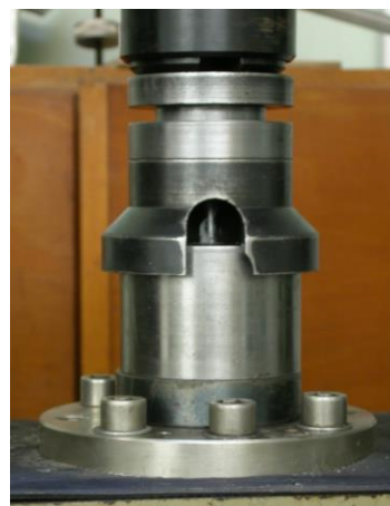
Fig. 4: The die set for backward extrusion
