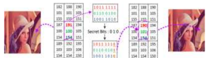
Figure (1): Basic 1-bit LSB embedding mechanism
