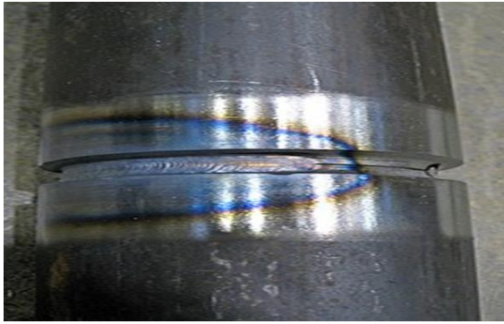
Figure 14 - Oxidation Dark Blue Surface of HAZ [1].
