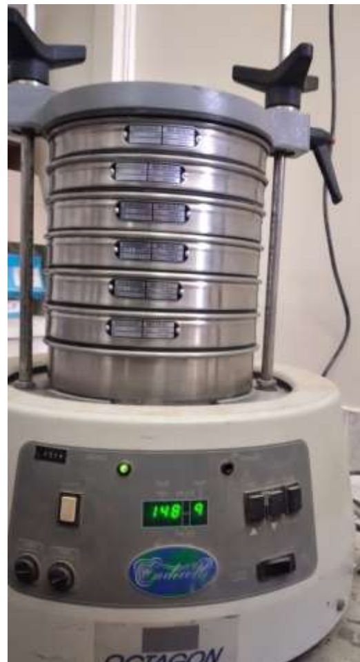
Fig. 1. Sieves and Shaker used for fillers preparation.
