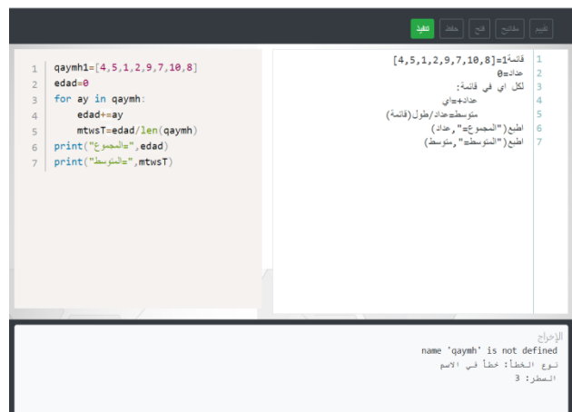
Figure 6. Sample 2: ArPy with output error handling
