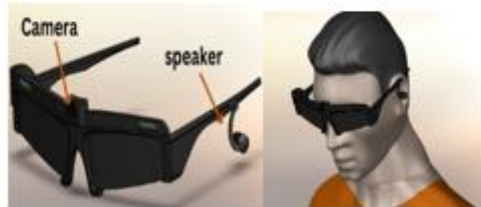
Figure 2: Smart Glasses Model for the Proposed System.
