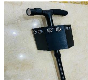
Figure 5: Smart Stick with Three Ultrasonic Sensors for the Proposed System.
