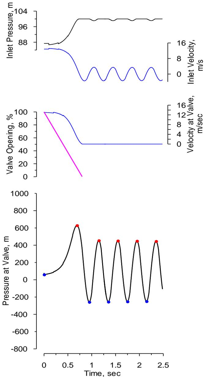
Figure 3. Pressure Transient Without Valve Oscillatory
