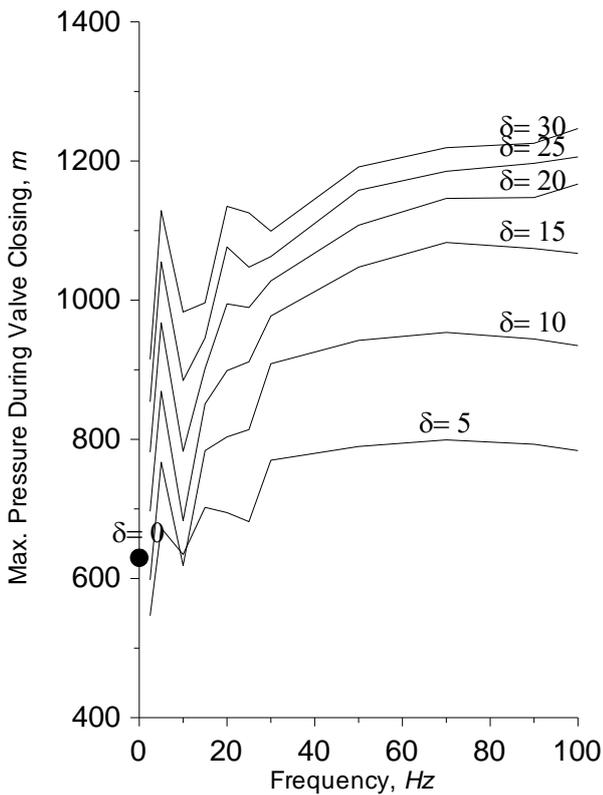
Figure 9. Transient Max. Pressure for Different Altitude and Frequency
