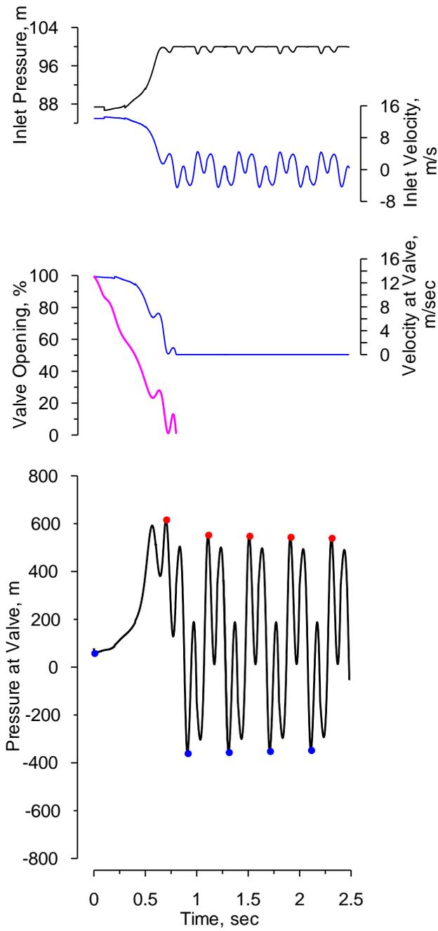
Figure 5. Pressure Transient  $\delta=10^\circ$ ,  $f=10$  Hz
