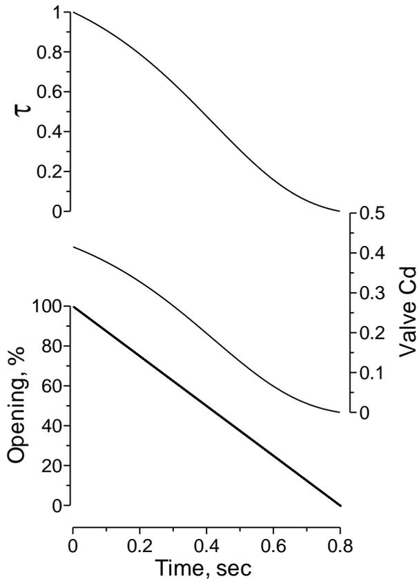
Figure 1. Valve Closing Characteristics Without Oscillatory
