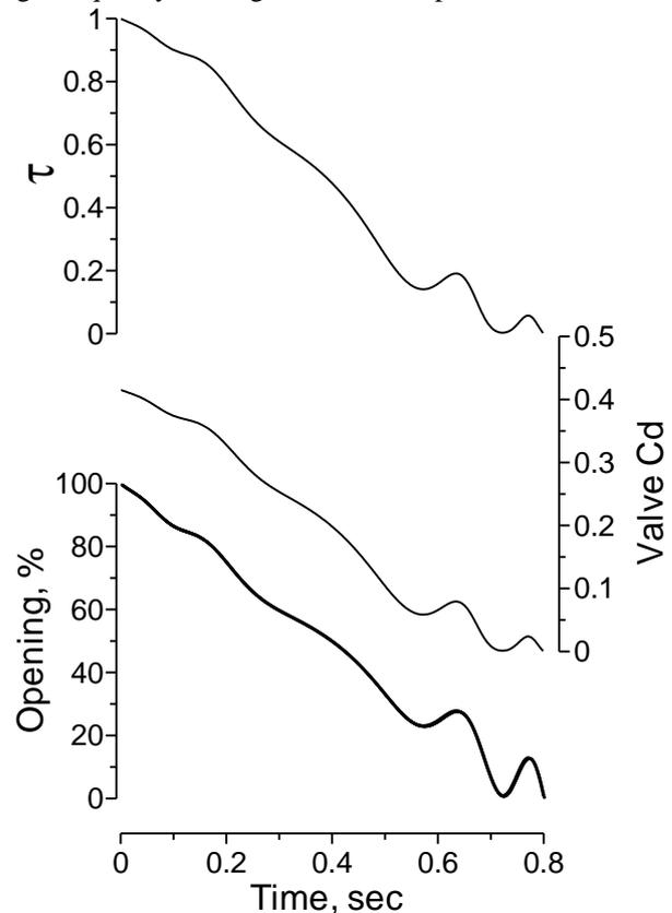
Figure 2. Valve Closing Characteristics  $\delta=10^\circ$ ,  $f=10$  Hz
