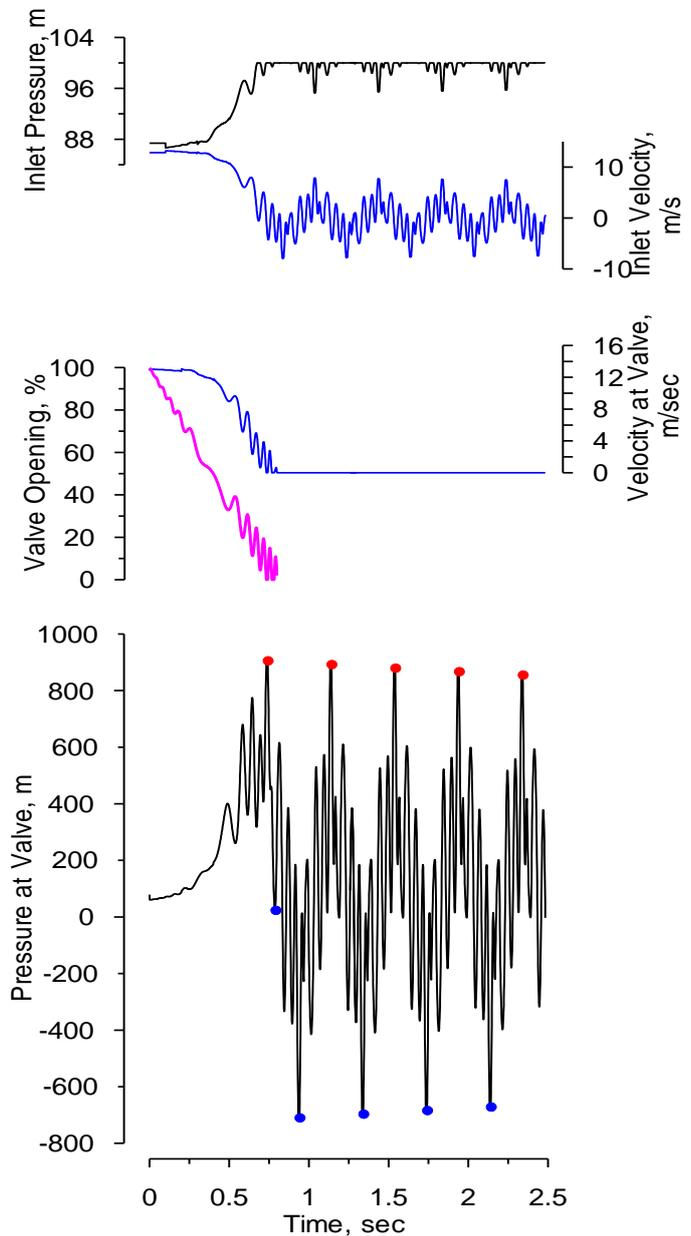
Figure 4. Pressure Transient  $\delta=10^\circ$ ,  $f= 30$  Hz
