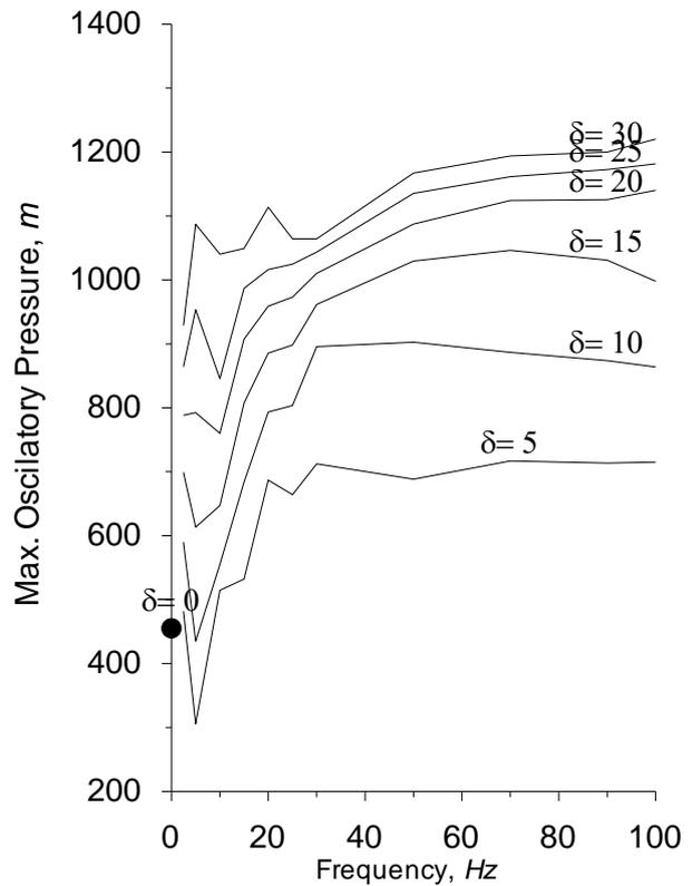
Figure 10. Oscillatory Max. Pressure for Different Altitude and Frequency
