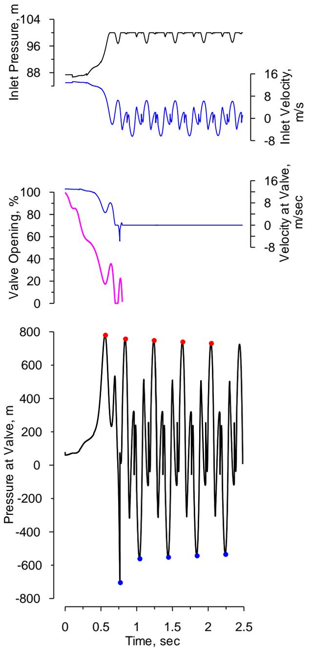
Figure 6. Pressure Transient  $\delta=20^\circ$ ,  $f=10$  Hz
