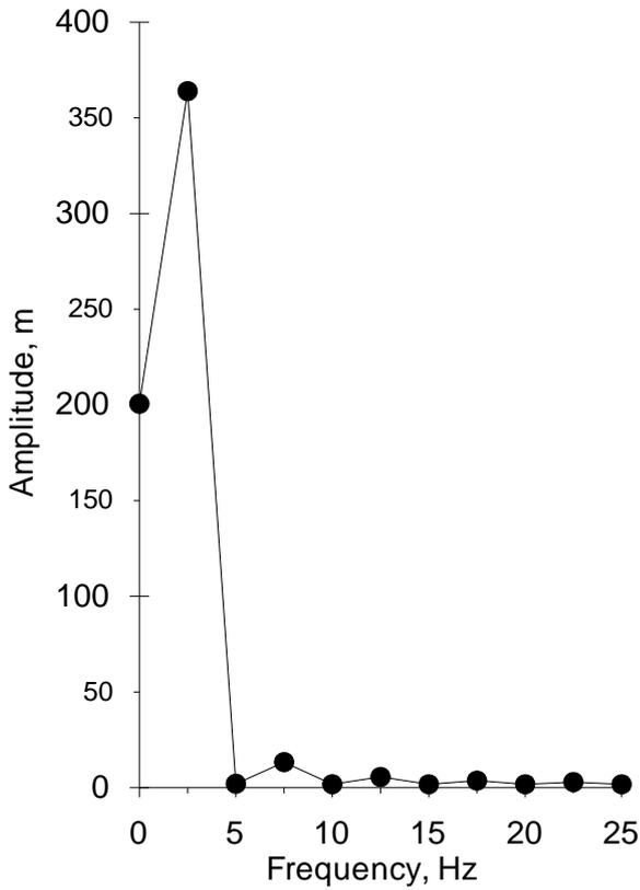
Figure 7. Pressure Spectrum Without Valve Oscillation
