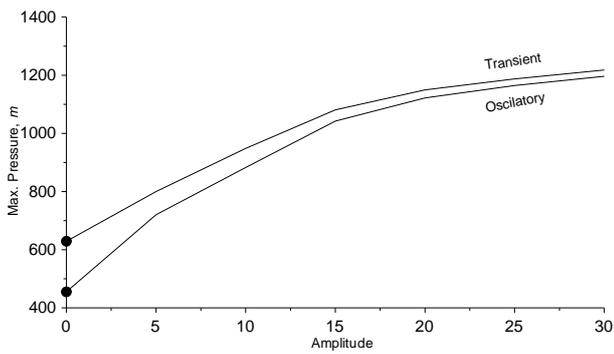
Figure 11. Asymptotic Oscillatory and Transient Maximum Pressures at Different Amplitude
