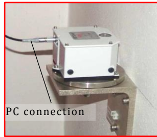
Figure 3. Inclinometer - Leica Nivel 210
