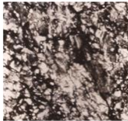
Figure 17. The Surface of Electrochemically Dissolved Copper Objective Epi 8/0.15/, (Anode).
