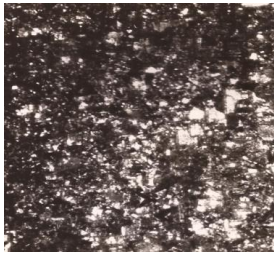
Figure 15. The Surface of Deposited Copper. /Objective Epi 8/0.15/, Current Density -100 \text{ A/m}^2 , Temp. -40^\circ\text{C} . gelatin -10 \text{ ppm} .
