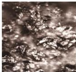
Figure 9.The Surface of Deposited Copper. /Objective Epi 8/0.1./, Current Density – 400 A/m 2 , Temp. – 65 0 C.
