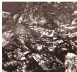
Figure 10. The surface of deposited copper. /Objective Epi 8/0.15/, Current density – 400 A/m 2 , Temp. – 40 0 C. gelatin – 10 ppm.
