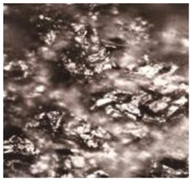
Figure 8 . The Surface of Deposited Copper. /Objective Epi 8/0.15/, Current Density – 400 A/m 2 , Temp. –50 0 C.
