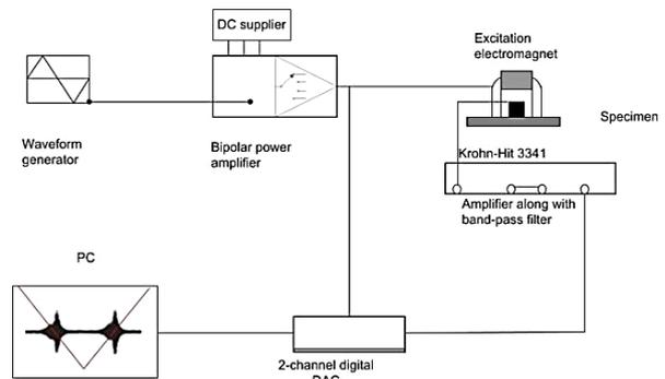
Figure. 2. Schematic Layout of the MBN Measurement Apparatus
