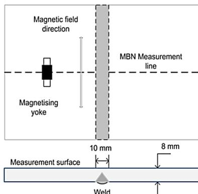
Figure. 1. Schematic Layout of the MBN Measurement Setup
