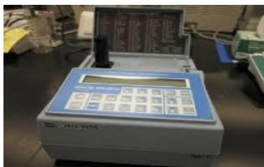
Figure 5. Model HACH DR 2010 Spectrophotometer
