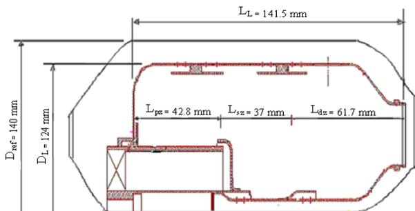
Figure 1. Chamber Main Dimensions.
