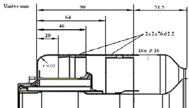
Figure 5. Secondary Zone Airflow Distribution.
