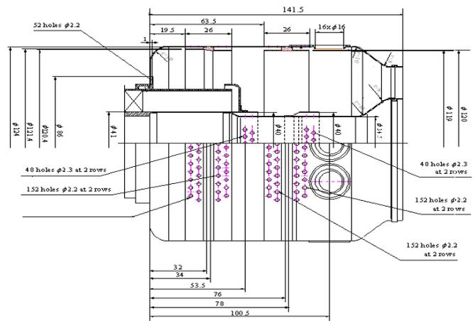
Figure 10. Combustion Chamber Dimensions and Air Distribution Summary.
