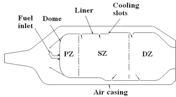
Figure 2. Combustion Chamber Zones.
