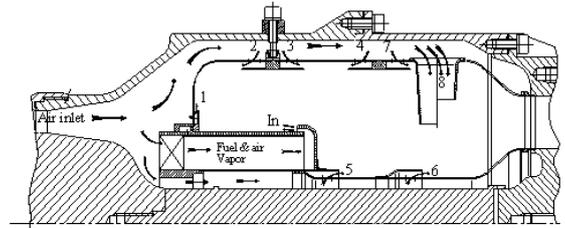
Figure 9. Air Admission Holes Location.
