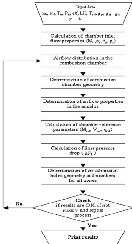
Figure 8. Physical Model Program Flow Chart.
