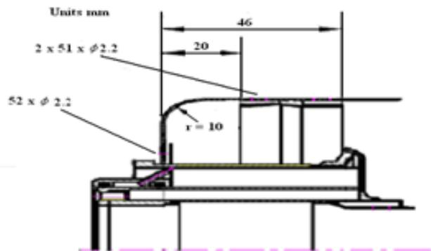
Figure 4. Primary Zone Airflow Distribution.
