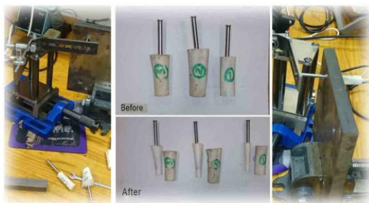
Figure 4. Positive results with pig bones encasing the cement and implant positioned at optimum pivotal distance and exposed to optimal frequency of vibration.
