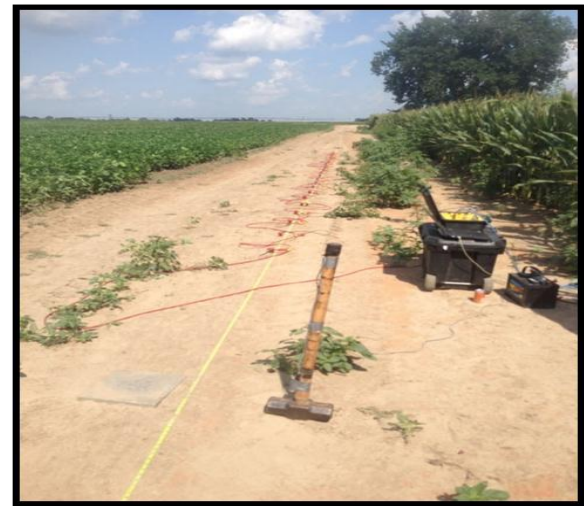
Figure 8. Location of the shot points for MASW array line.
