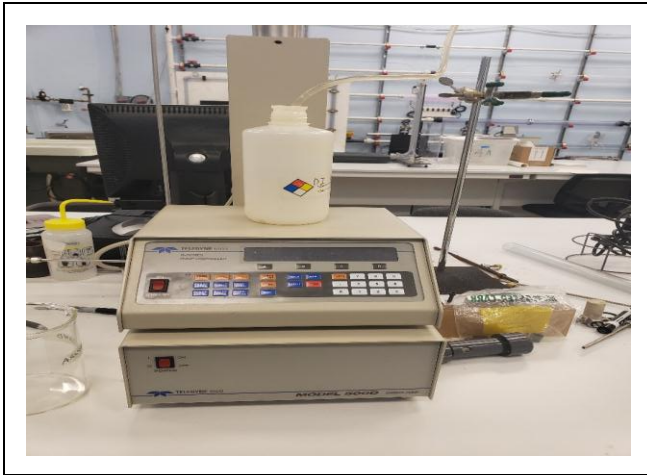
Figure 4. Showing the Syringe Pump
