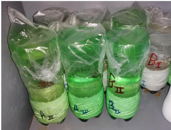
Figure 5: The experimental setup for chloride penetration test
