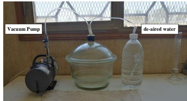
Figure 2: Vacuum saturation apparatus setup
