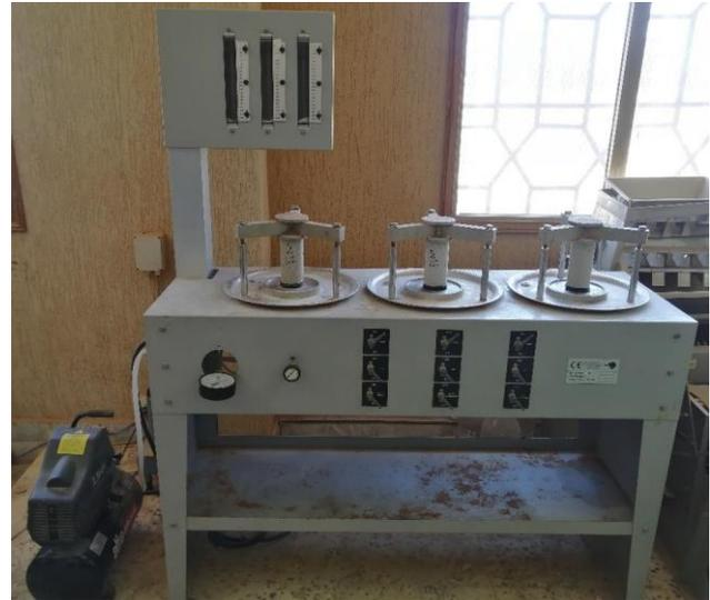
Figure 4: water permeability apparatus setup
