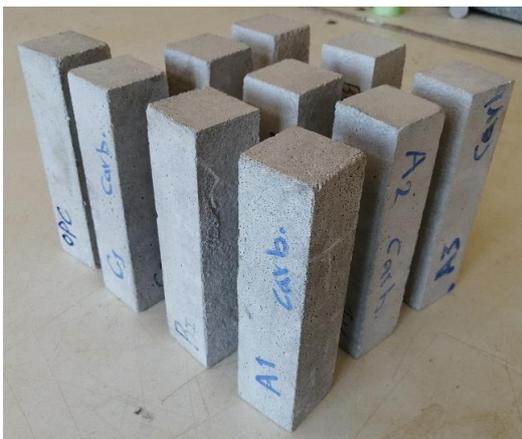
Figure 6: Exposure to natural carbonation (laboratory environment)
