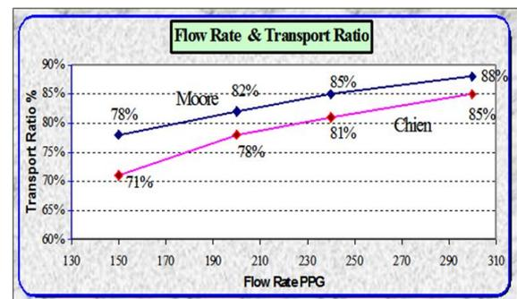
Figure. (5) Relationship between the flow Rate and Cutting Transport Ratio in Moore and Chien.
