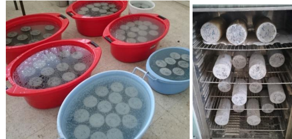
Figure 3. Curing condition a) in solution (0,5,10,15% NaCl; b) in oven of 60°C.
