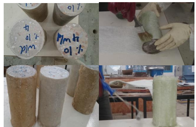
Figure 4. Covered column with GFRP.
