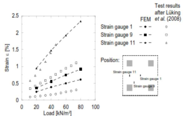
Figure 9. Comparison of measured and calculated strains
