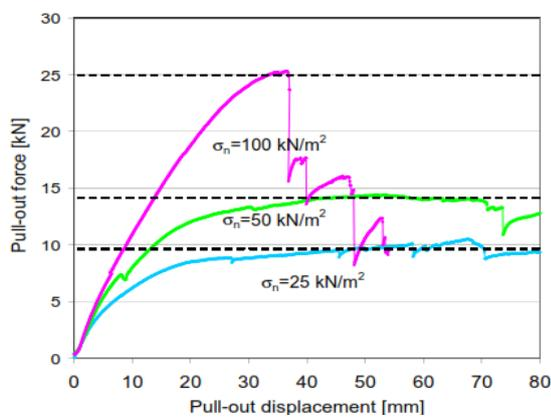
Figure 7. The load-displacement relationships
