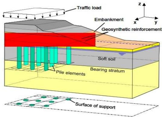
Figure 2. Geosynthetic-reinforced pile-supported embankment
