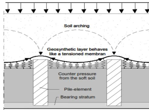
Figure 3. Mechanisms of load transfers
