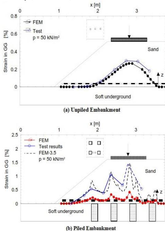
Figure 10. Strain in reinforcement
