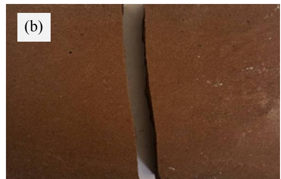
Figure 17. Images for the fracture mode of floor ceramic tiles
