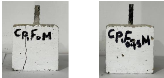
a) CPF0 b) CPF0.75 Figure. 19 Sample after exposed to 10% magnesium (120 days)
