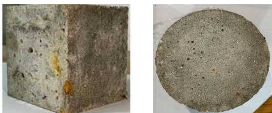
Figure 15. Sample after exposed to 10% magnesium (120 days)
