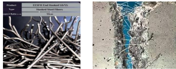
Figure 3. Steel fibers added to Concrete
