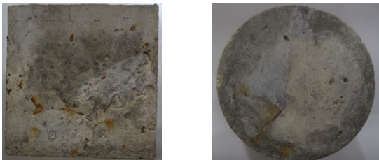
Figure 14. Sample after exposed to 10% magnesium (60 days)
