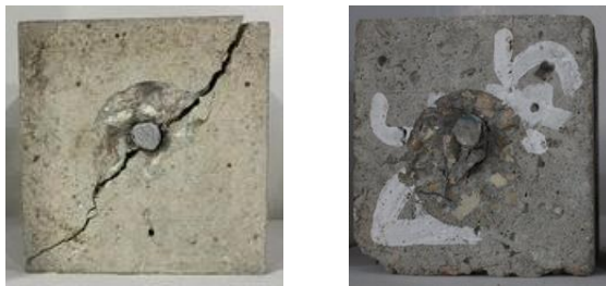
a) CPF0 b) CPF0.75 Figure. 18 Control sample (no exposure)
