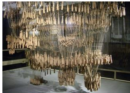
Figure 1. Antonio Gaudi, Reproduced Model of “La Sagrada Familia”, 1983-1926. Up Side down Structural Analysis Made from Strings and Weighted Sacks.
