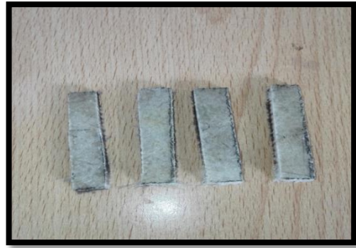
Figure 8-b. Woven Roving Impact Test Specimens.
