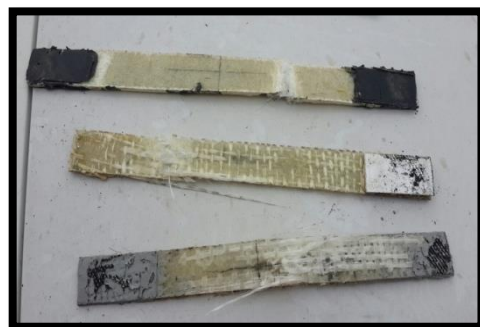
Figure 12. Failed Specimens by the Tensile Test.
