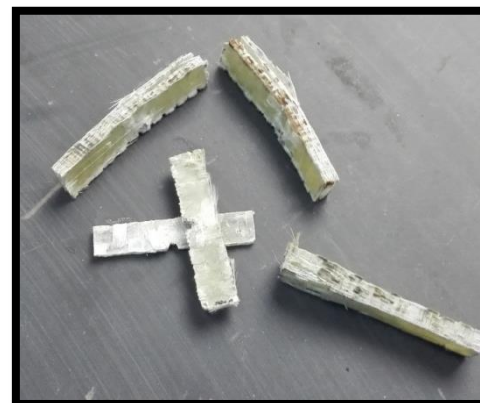
Figure 12. Failed Specimens by the Tensile Test.
