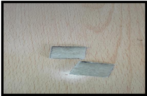
Figure 7- b. Chopped Mat Hardness Test Specimens.
