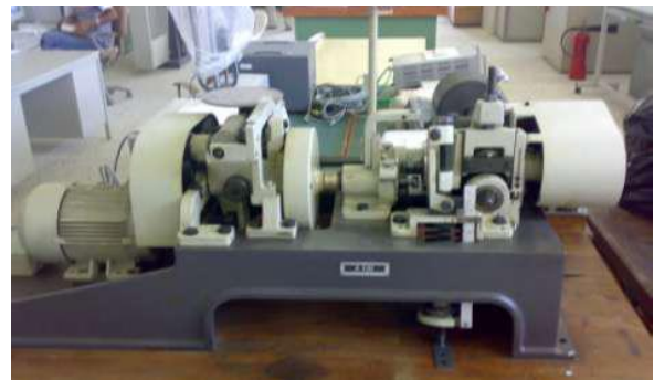
Figure 3. Block on Ring Wear Test Machine.
