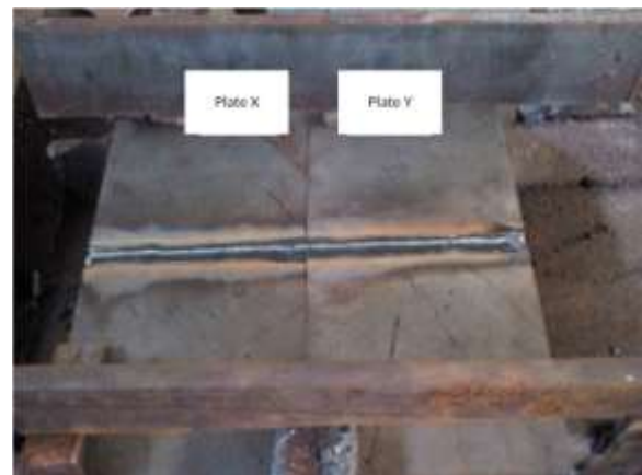
Figure 1. The Welded Plates.
