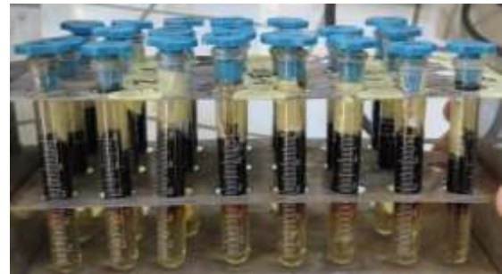
Figure 19: Results of Different Salinity with SDS Surf. 0.15 and CTAB Surf 1.5 at 50 °C.
