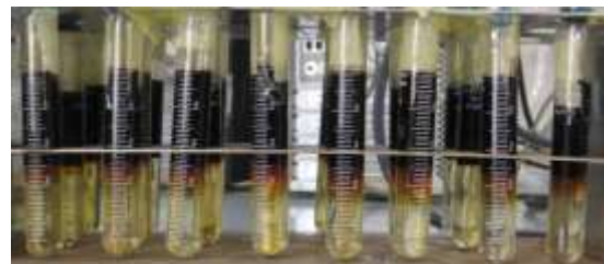
Figure 13: Results of Different Salinity with SDS Surf. 0.1 and CTAB Surf 1 at 50°C
