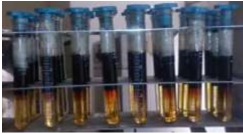
Figure 15: Results of Different Salinity with SDS Surf. 0.1 and CTAB Surf 1 at 70°C.
