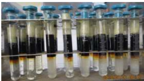
Figure 23: Results of the Different Salinity with SDS Surf. 0.2 and CTAB Surf. 2 at 30 °C
