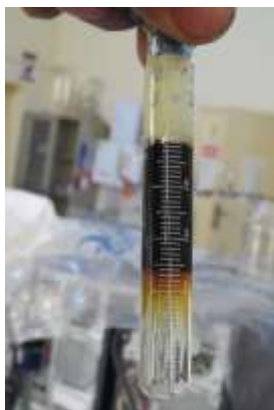
Figure 5: Results of Different Salinity with SDS Surf. 0.05 and CTAB Surf. 0.5 at 30°C.
