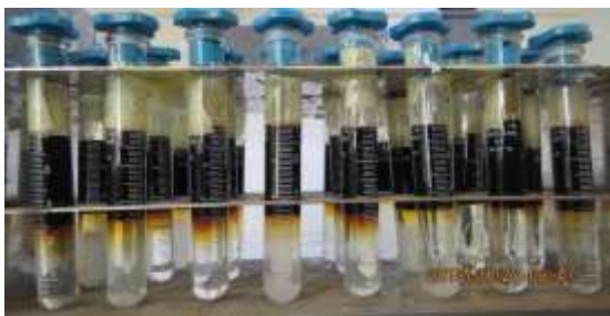
Figure 11: Results of Different Salinity with SDS Surf. 0.1 and CTAB Surf 1 at 30°C.
