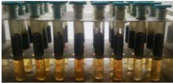
Figure 17: Results of Different Salinity with SDS Surf. 0.15 and CTAB Surf 1.5 at 70 °C.
