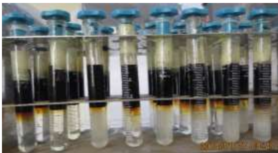
Figure 17: Results of Different Salinity with SDS Surf. 0.15 and CTAB Surf 1.5 at 30 °C.
