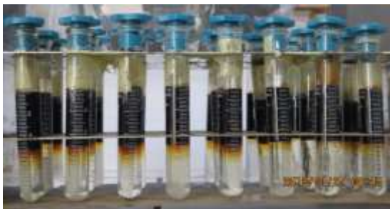
Figure 4: Results of Different Salinity with SDS Surf. 0.05 and CTAB Surf. 0.5 at 30°C.
