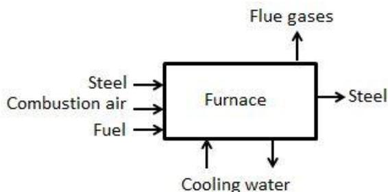
Figure 2. Schematic of the Parameters Considered in Performing the Overall Heat and Material Balance.
