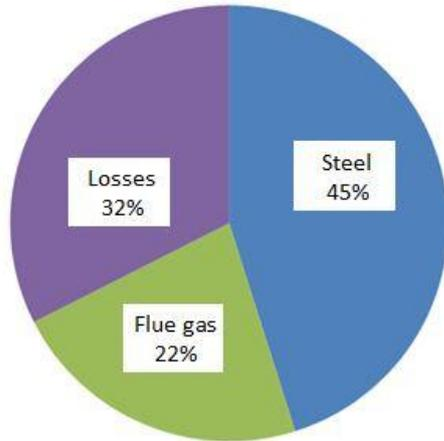
Figure 4. Output Energy Distribution in the Reheating Process of Steel Billets in the Reheat Furnace.
