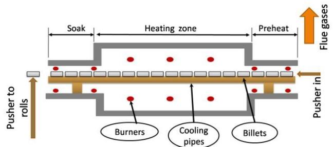
Figure 1. Side View of Pusher Type Steel Billet Reheat Furnace at Libyan Iron and Steel Company (LISCO).
