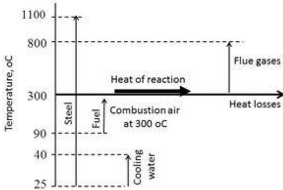
Figure 3. Schematic of the Parameters Considered in Performing the Overall Heat Balance.
