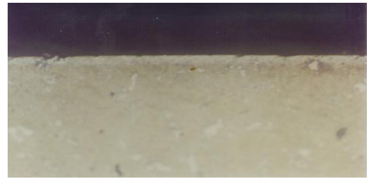
(a)Heat treated grinding white layers
