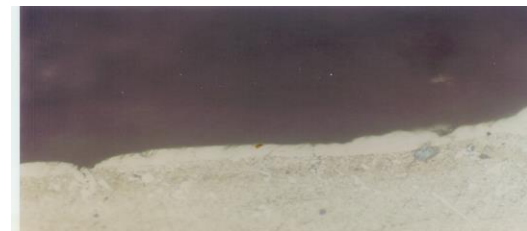
(b) Hard turning white layer.
