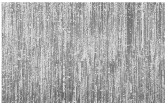
(b) Surface generated under the hard machining technique (1000x)
