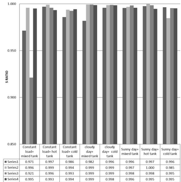
Figure 6. Entropy ratios for all manifolds under all test conditions
