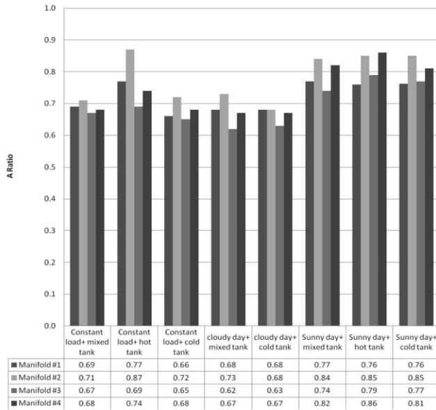
Figure 5. Exergy ratios for all manifolds under all test conditions
