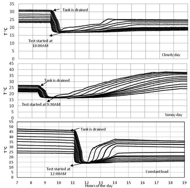
Figure 7. Stratification performance of Manifold #2 under cold tank condition (the constant temperature lines from the bottom to the top in the figure correspond to the temperature readings obtained from the bottom to the top of the tank)
