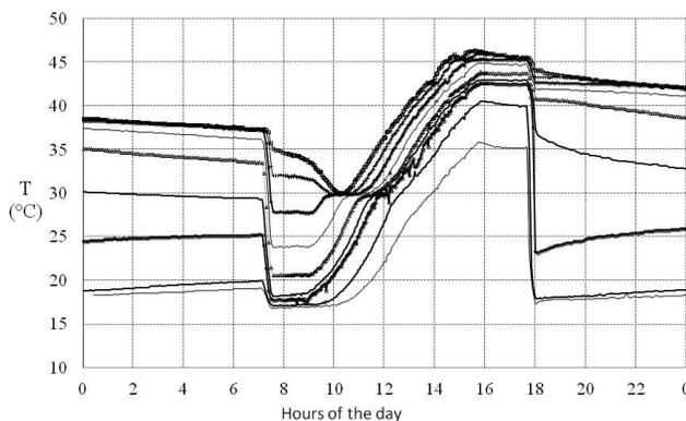
Figure 1. Temperature distribution in the SDHW tank using Manifold #1 (the constant temperature lines from the bottom to the top in the figure correspond to the temperature readings obtained from the bottom to the top of the tank)
