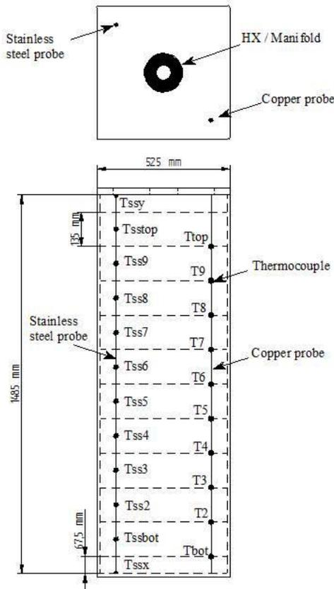
Figure 4. Locations of thermocouples on the two probes.
