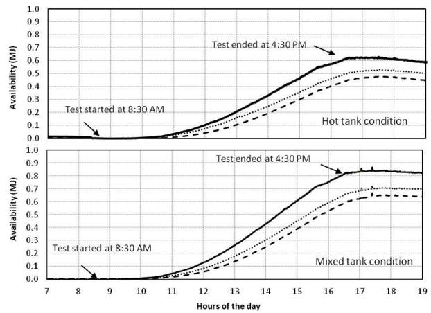
Figure 10. Availability ratio for sunny day condition with Manifold 2.
