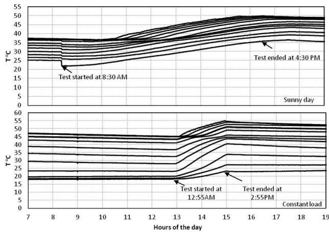
Figure 8. Stratification performance of Manifold #2 under hot tank condition (the constant temperature lines from the bottom to the top in the figure correspond to the temperature readings obtained from the bottom to the top of the tank)
