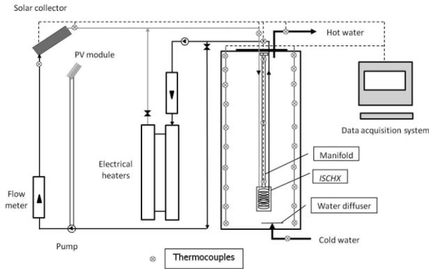
Figure 3. Schematic diagram of the experimental set-up
