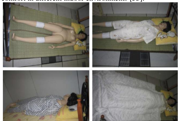
Figure 6. examples of experiment of sleeping conditions with different level of clothing insulation. Source: Lin (2008)
