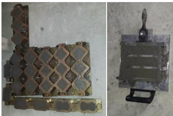
Figure 6 Mortar Specimens in Moulds
