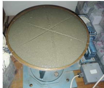
Figure 7 Flow Test of Mortar
