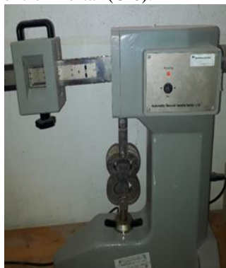
Figure 10 Mortar Specimens under Direct Tensile Test
