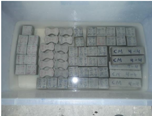
Figure 5 Mortar Specimens in Curing Water
