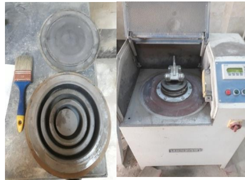
Figure 4 Ring mill used to grind slag to required fineness
