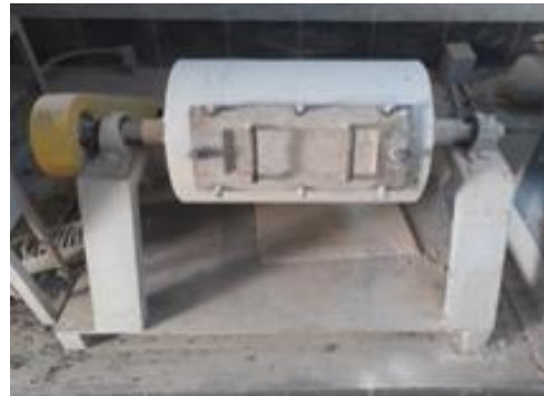
Figure 3 Ball mill used to grind slag aggregates
