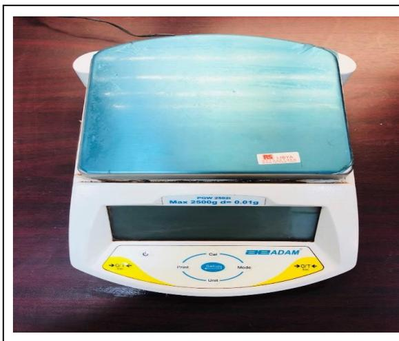
Figure 5. Electronic scale
