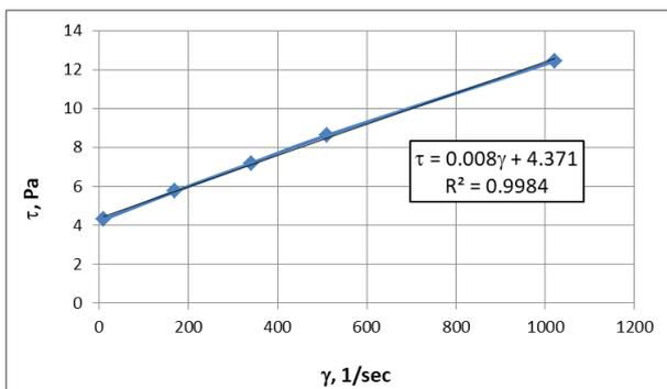
Figure 15. Shear stress vs. shear for Test # 4
