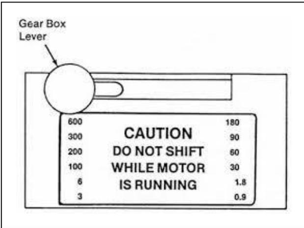
Figure 8, b. Speeds of Fann Model 35 Viscometers
