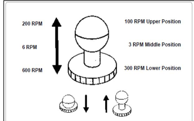
Figure 8, c. Speeds of Fann Model 35 Viscometers
