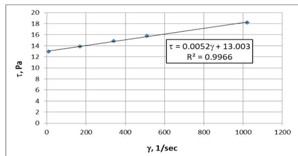
Figure 12. Shear stress vs. shear rate for Test # 1
