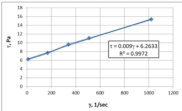
Figure 14. Shear stress vs. shear rate for Test # 3
