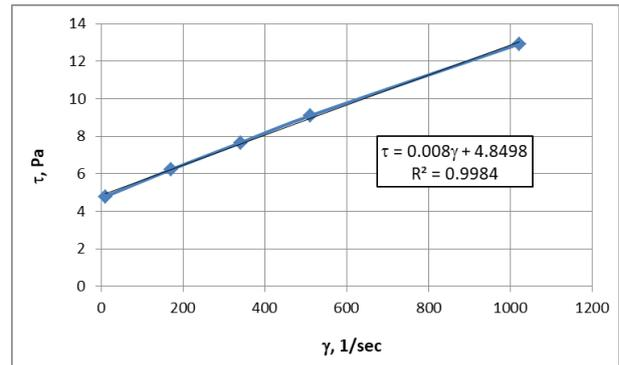
Figure 16. Shear stress vs. shear rate for Test # 5
