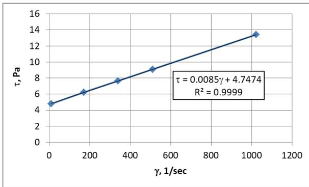
Figure 13. Shear stress vs. shear rate for Test # 2
