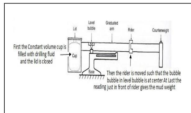
Figure7. Components Mud Balance
