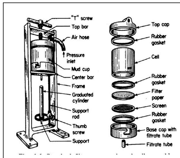
Figure 9. Standard API Filter Press
