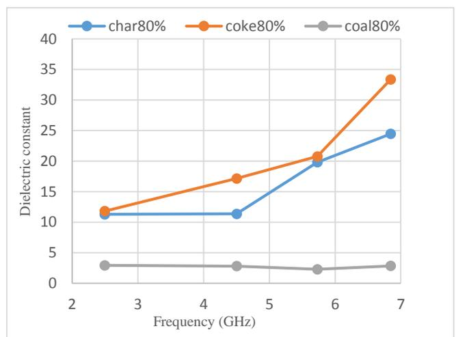
Figure 11. Real components of complex permittivity of lab-made samples
