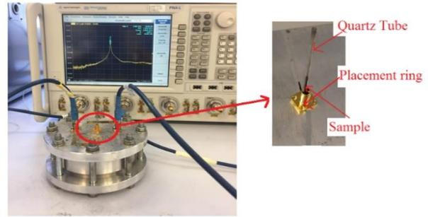
Figure 2. Photographs of the experiment set-up for cavity perturbation measurement.
