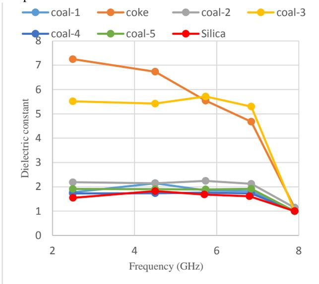
Figure 7. Real components of complex permittivity of different types of carbons
