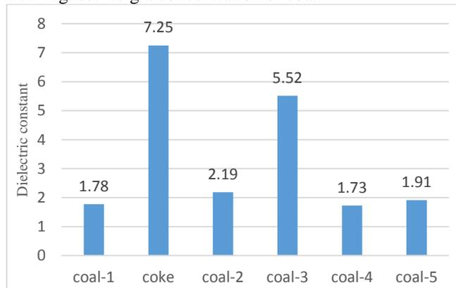
Figure 3. Dielectric constant of different carbon samples. The typical standard error is  $\pm 0.03$ , which in most cases is too small to observe.
