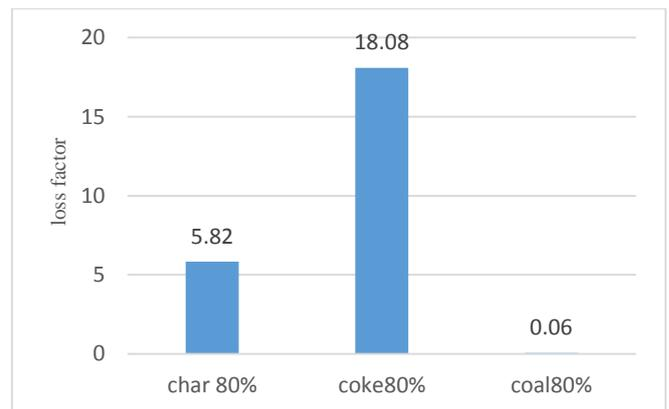
Figure 6. Dielectric loss factor of lab-made carbon samples. The typical standard error is  $\pm 0.024$ , which in most cases is too small to observe.
