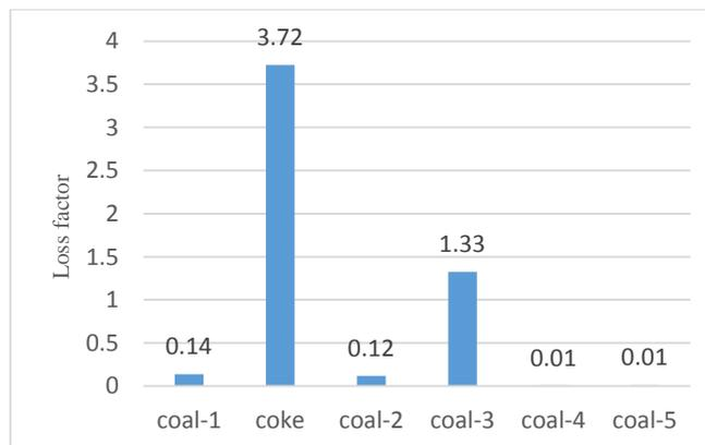
Figure 4. Dielectric loss factor of different carbon samples. The typical standard error is  $\pm 0.03$ , which in most cases is too small to observe.
