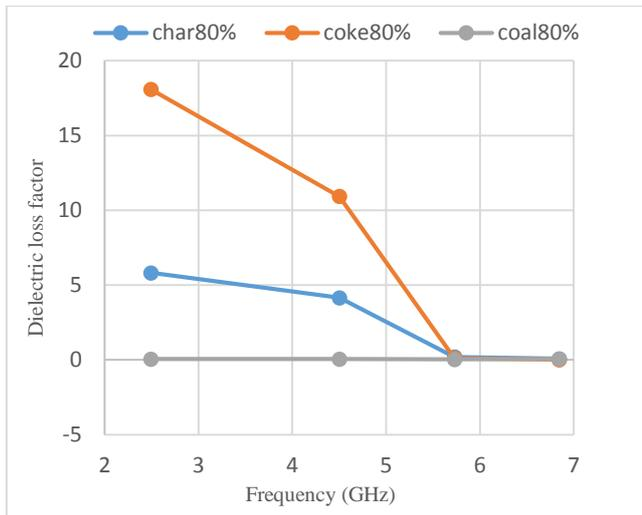
Figure 12. Imaginary components of complex permittivity of lab-made samples
