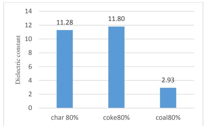
Figure 5. Dielectric constant of lab-made carbon samples. The typical standard error is  $\pm 0.01$ , which in most cases is too small to observe.
