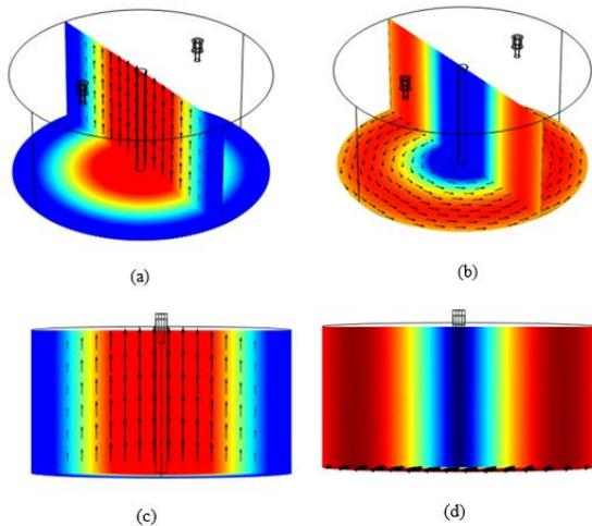
Figure 1 COMSOL simulation of the cylindrical cavity resonator  $TM_{010}$ , showing the electric ((a) and (c)) and magnetic ((b) and (d)) field distribution
