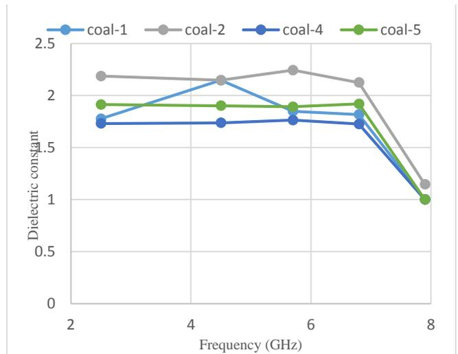
Figure 9. Real components of complex permittivity of different types of coals
