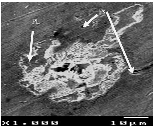
Figure 7 High magnification for the pits (P) showing the pitting interactions
